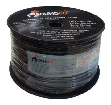
Soundco stereo cable model 4040 has two stereo cores with 28 copper strands, coated with polyethylene insulation in two colors, white and red. 64 all-copper shielded strands around each core strand in each line form a double-line cable with an outer PVC insulation cover.
